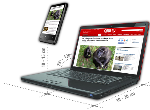
Figure 4: Parameters of reliability setup for initialization – distance between mobile device and laptop, range of screen angles used during tests and height range of a mobile device in order to be focused on the same point on the screen.
